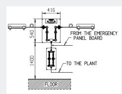
THE FIRST STAGE panel board develops an initial reduction of the pressure cylinder to a 12 bar pressure.
